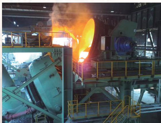
BSSF slag processing technology capacity:1~3t/min suitable for BOF &EAF
