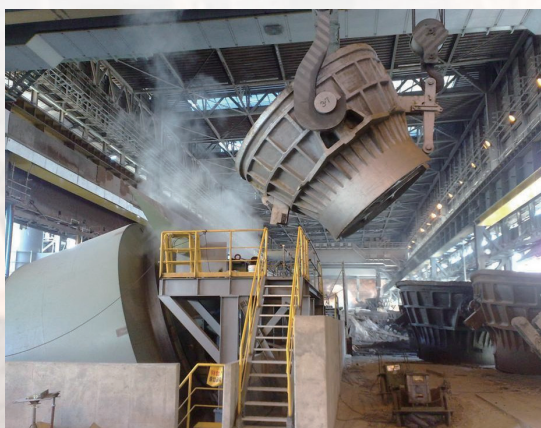
BSSF slag processing technology capacity:1~3t/min suitable for BOF &EAF
